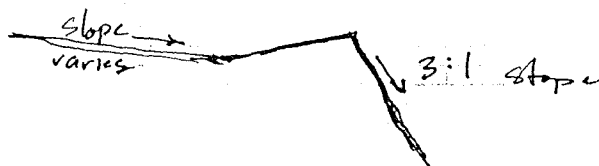
berm cross section
